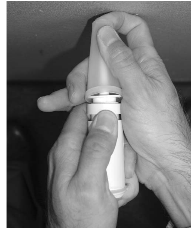
Step 3: Apply downward force with your thumb to create an opening 2/8 to 3/8" to view base of syringe tip and inspect for crack. Adjust angle to give best view of syringe tip.
